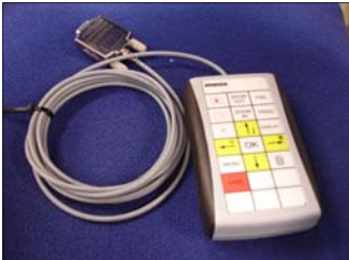
The new hand controller with integrated RS232 based control system
