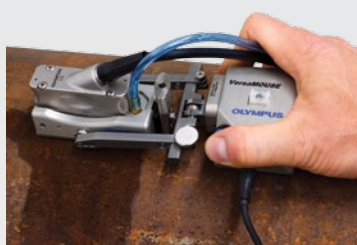
The RexoFORM and VersaMOUSE for one-line encoded scans, or 2-D mapping using the integrated indexing button.
