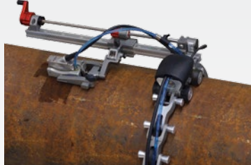
The RexoFORM and CHAIN Scanner for XY mapping of smooth pipes.
