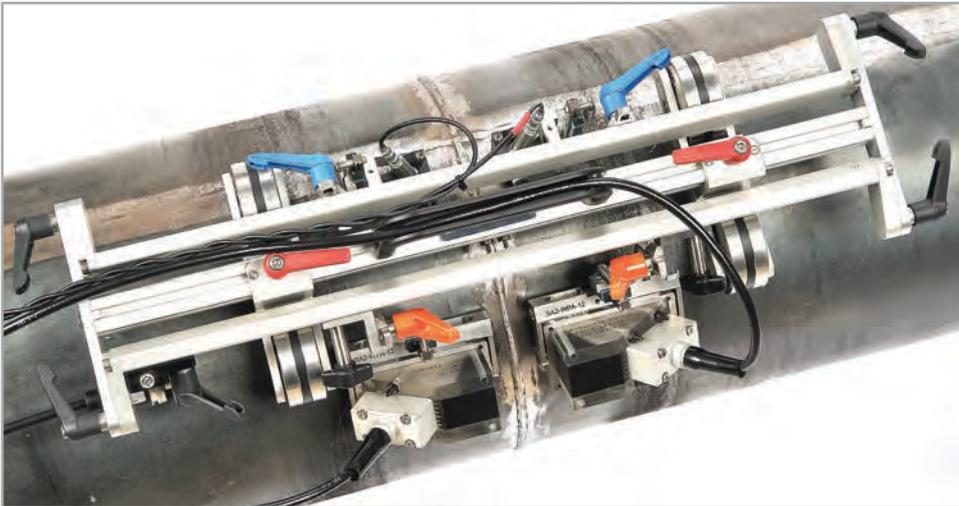
A highly versatile weld inspection manual scanner, ideal for use on pipes from 3" OD up to flat plate. MultiMag has magnetic wheels and is ideal for use with phased array, TOFD and pulse-echo techniques.
