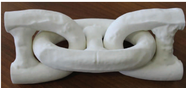
Corroded chain link model for geometry analysis, FEA and 3D printing
